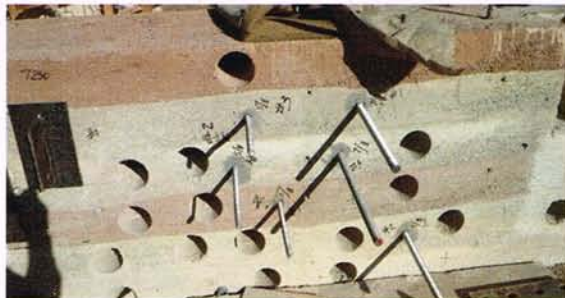
Trial walls were rammed on site and tested for compressive strength.
